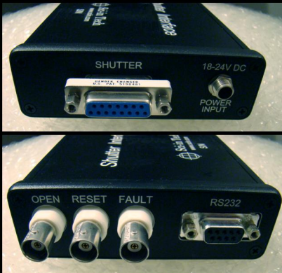
Shutter controller allows choice of operation. RS-232, contact-closure, USB with Opto-Isolator option.
