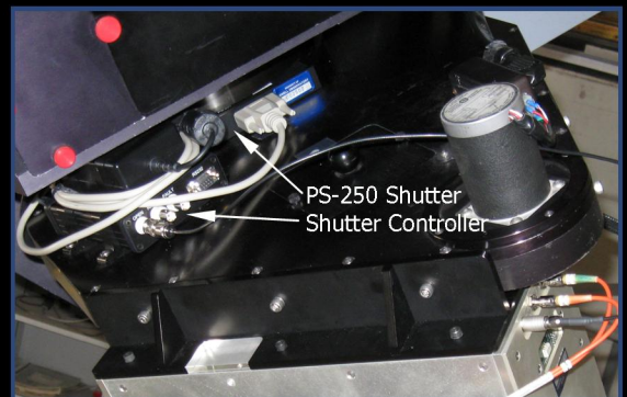
4Kx4K CCD camera for the 1.1-m Hall Telescope at Lowell Observatory
